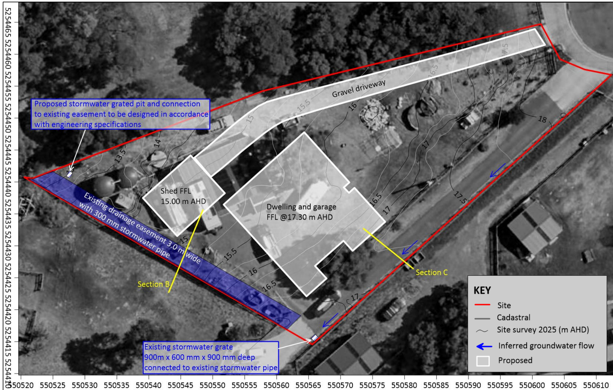
Map 3 Site plan showing drainage paths, proposed works, and
