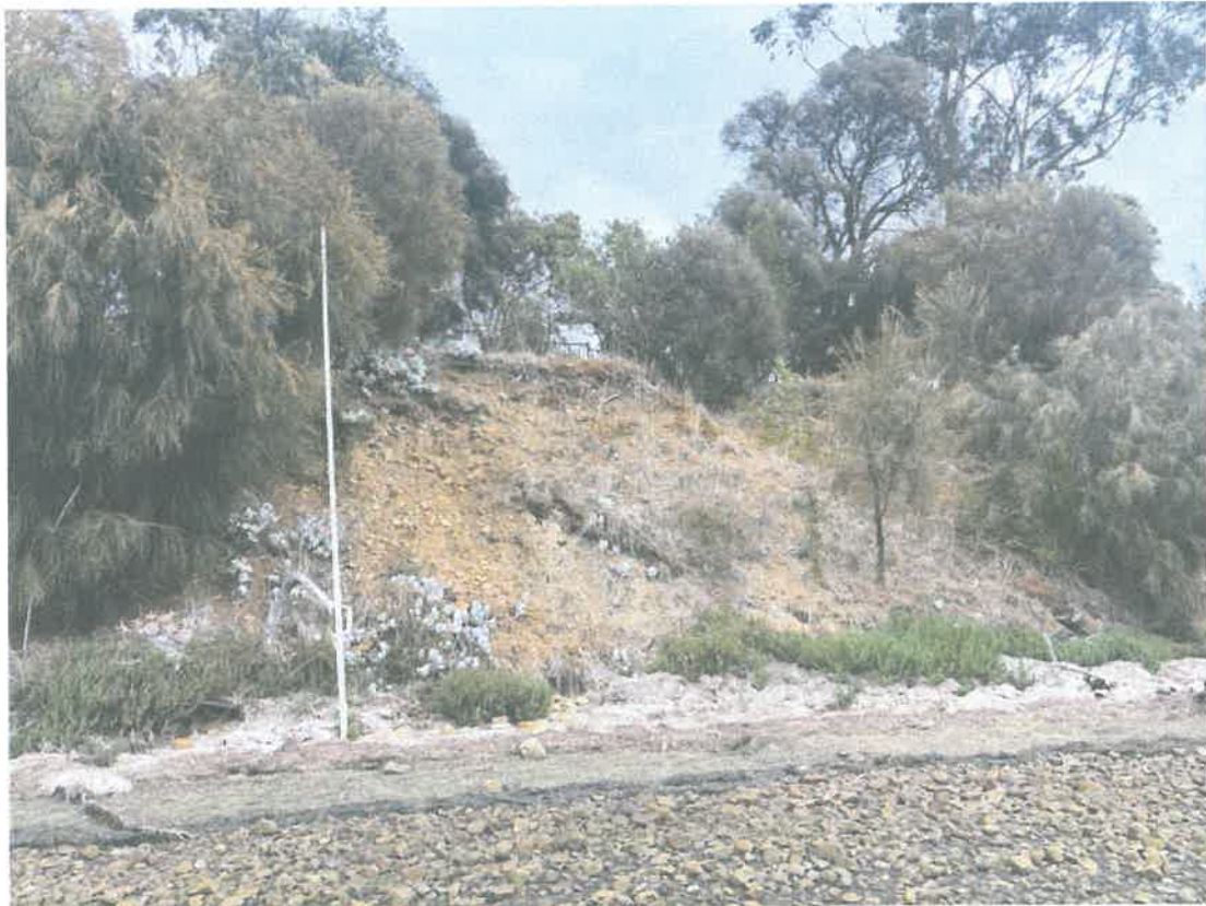
Plate 4. Tertiary-age sandy gravels occur on the coastal embankment bordering East Bay, about 50m south of 18 Imlay Street. Similar material may extend under the property. The staff is 5m high.
