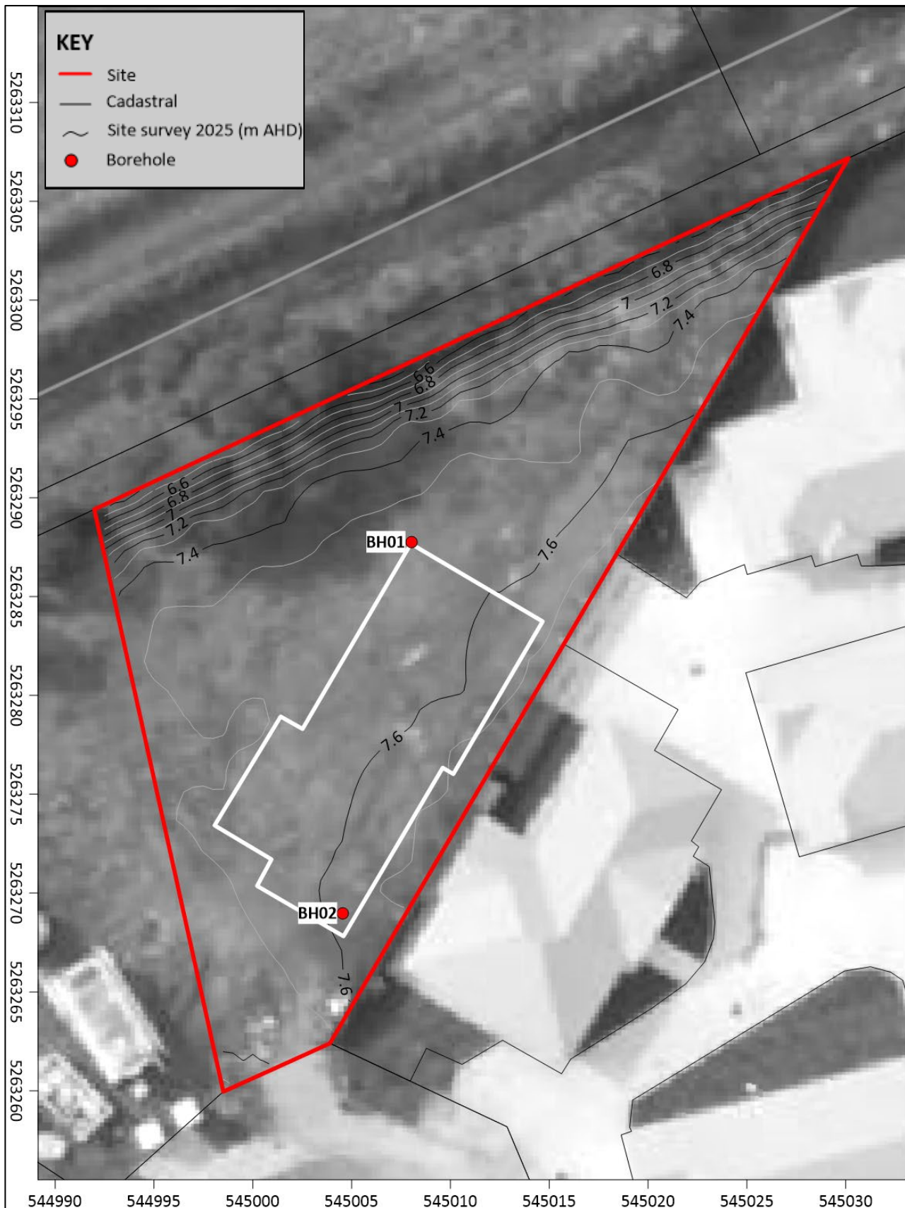
Map 5 Site plan and soil testing location
