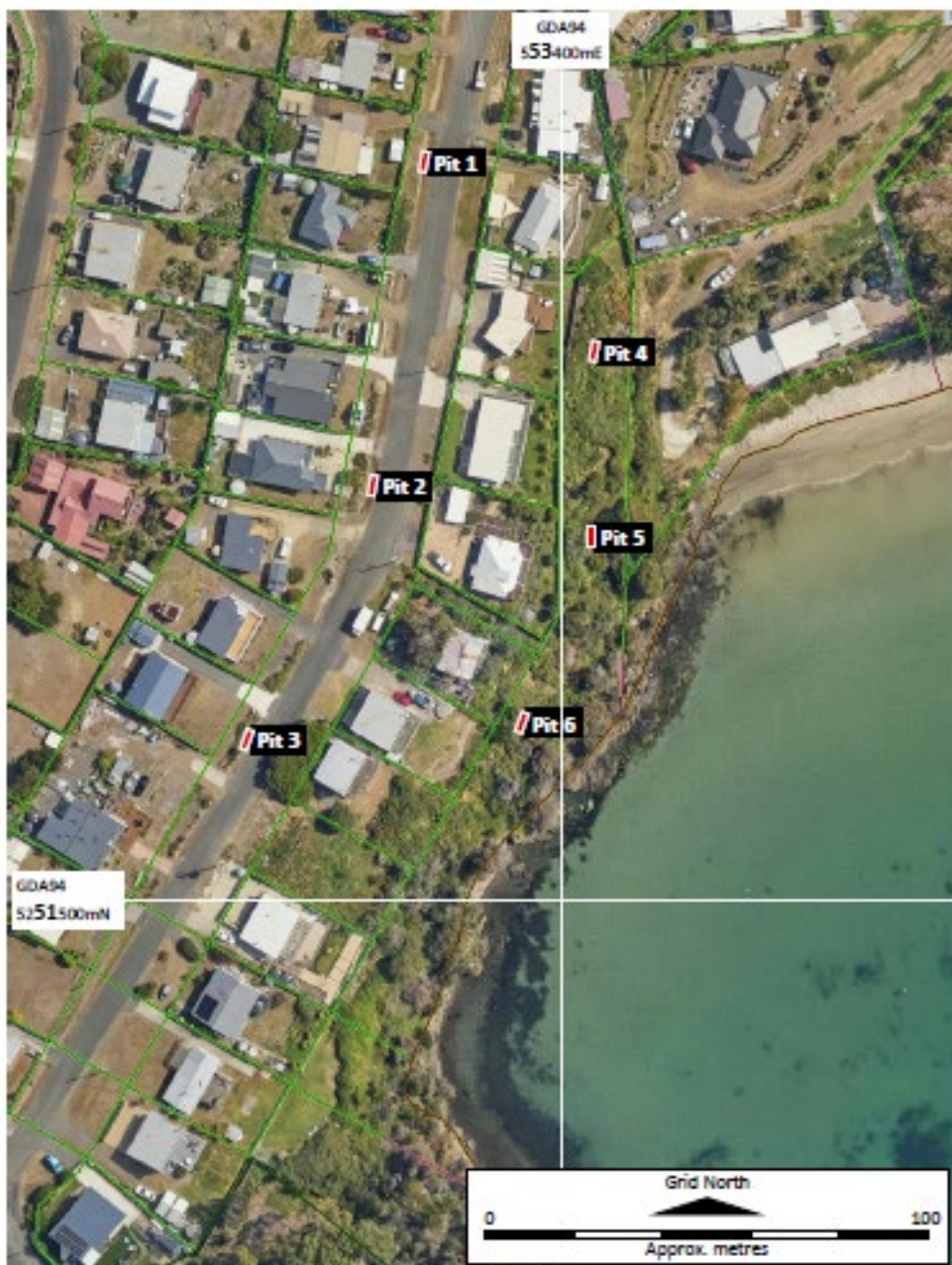
Figure 1. Proposed locations of six monitored excavator test pits in the vicinity of Carlton Bluff Road. These locations are nominal and may be amended after discussion between us, and by site conditions. Source: www.thelibrary.gov.au
