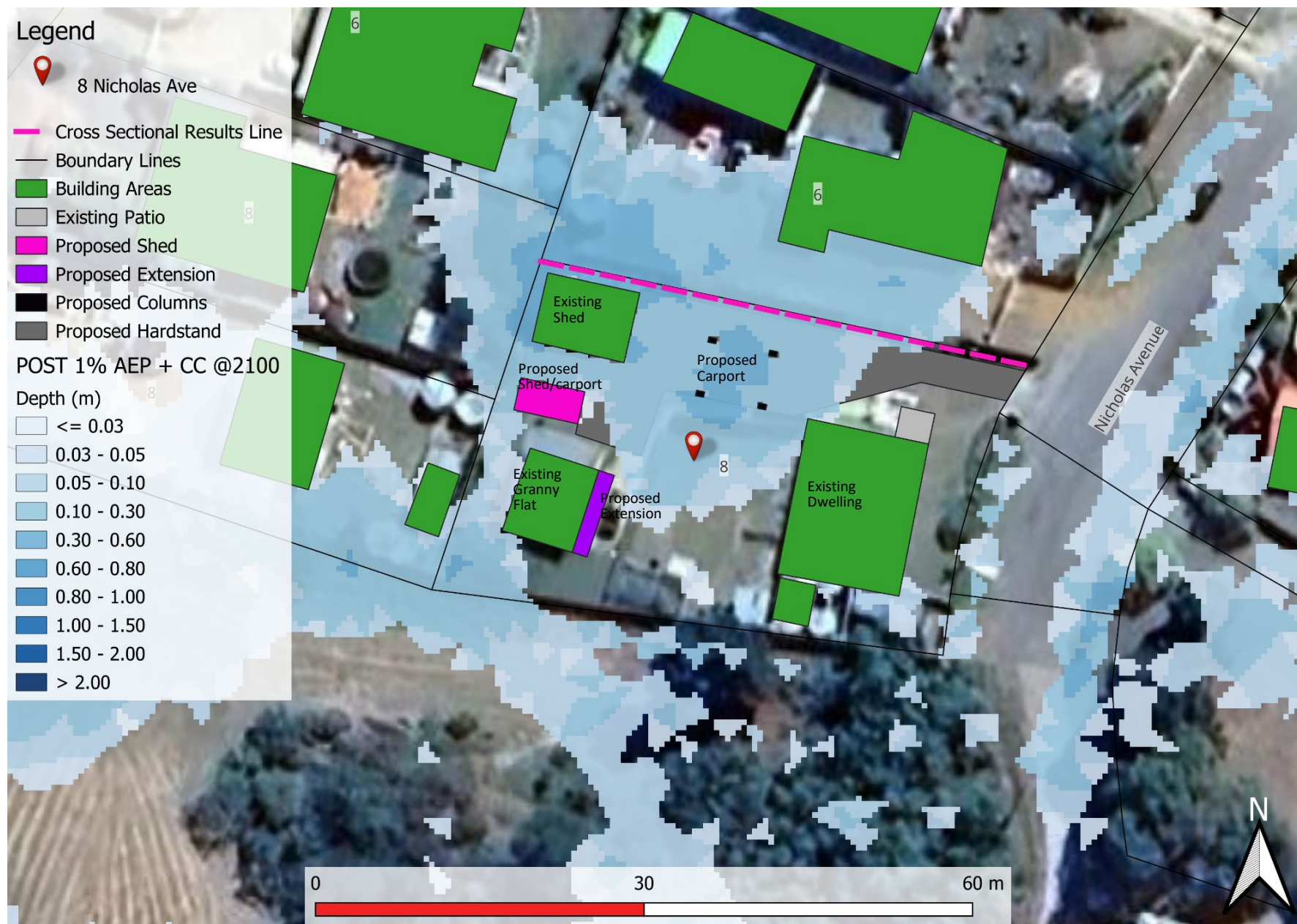
Figure 5. Post Development 1%+CC Flood Depth and extents
