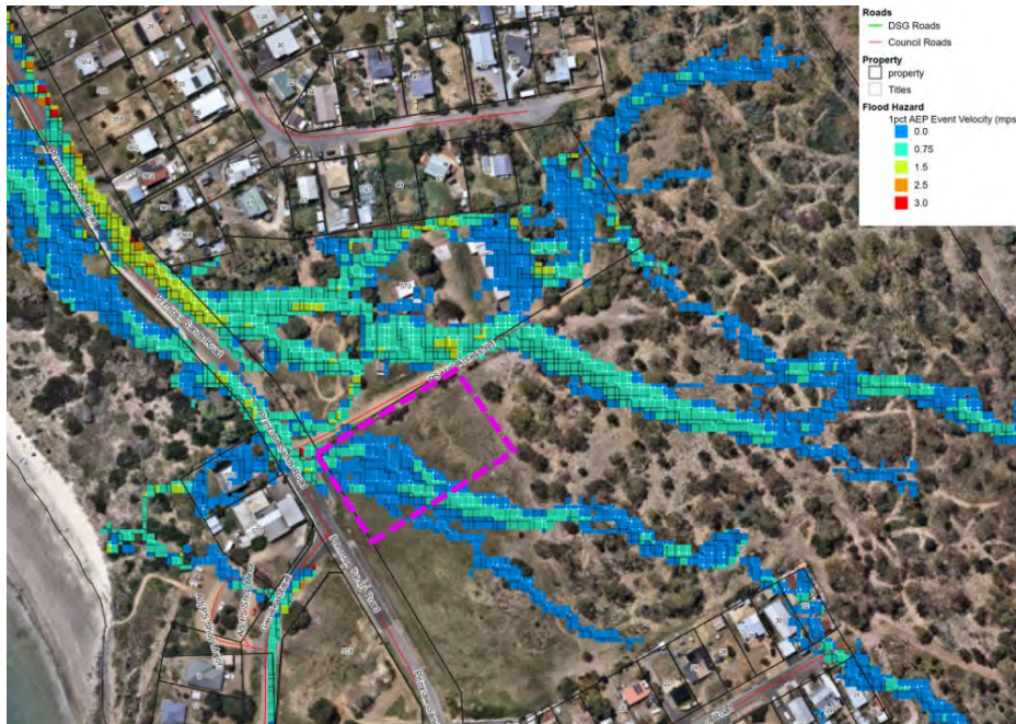
Figure 235: Flood Hazard Modelling of a 1%AEP flood event - velocity - with subject site identified. (source: Council supplied)
