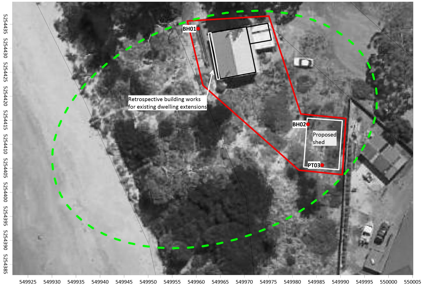
Figure 1 Site Borehole Locations
