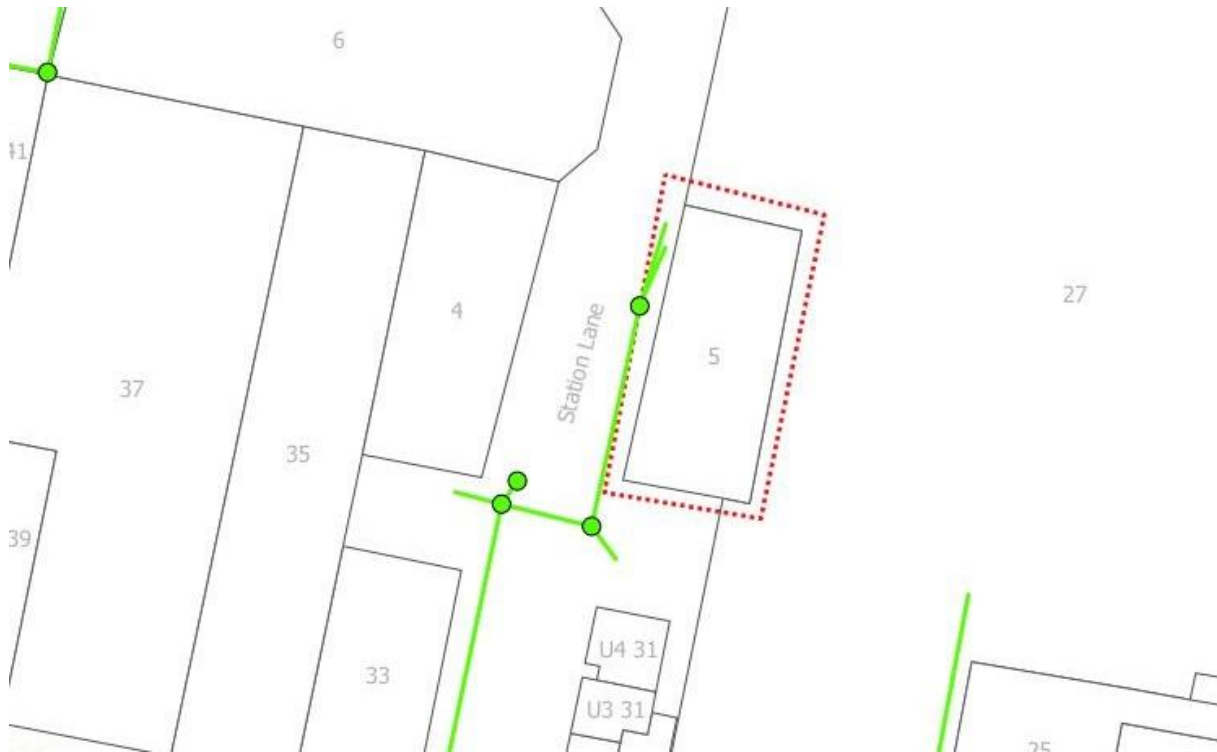
Figure 4: Sorell Council stormwater infrastructure around the site from DBYD records.
