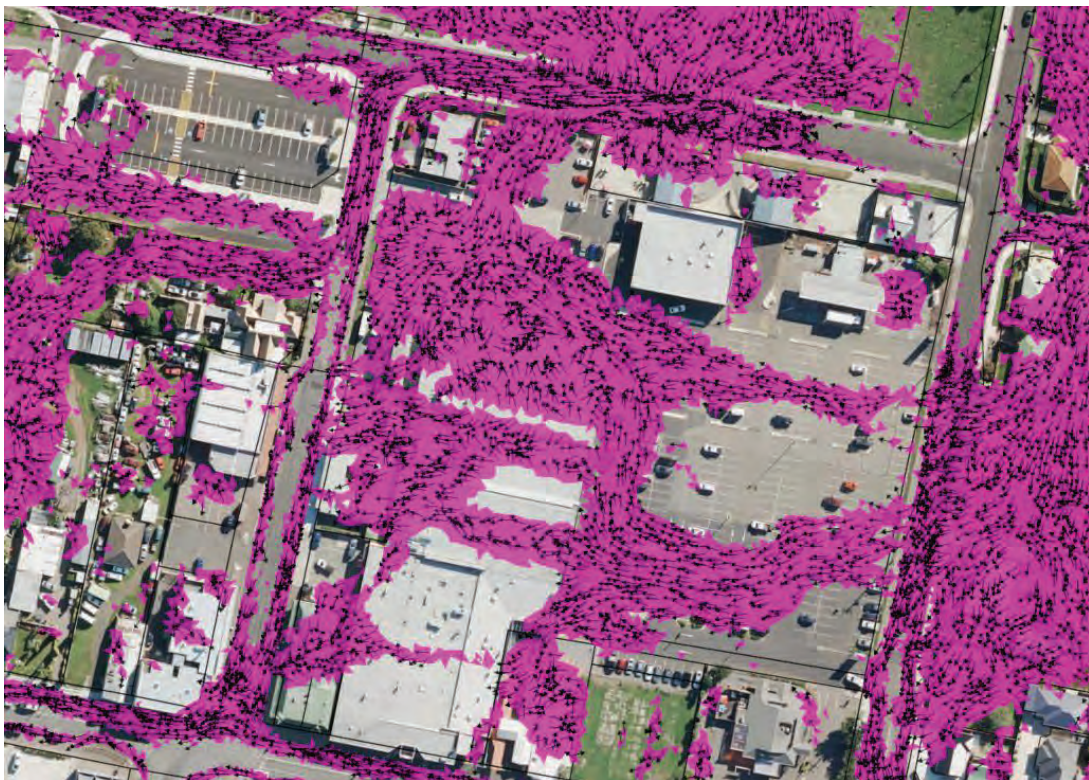
Figure 3. Indicative pre-development flow paths, resulting from a basic but conservative rain-on-grid model (depths >20mm)
