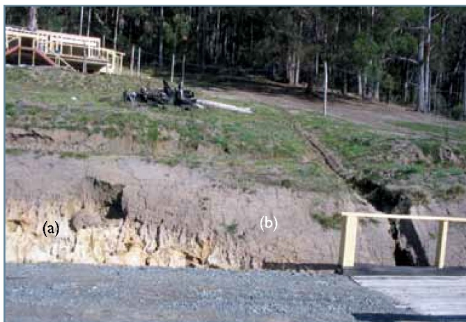
Figure 13. The severity (or sodium content) and depth of dispersive subsoils can vary considerably over short distances. (a). At this site highly dispersive subsoils exist meters away from (b) non-dispersive soils.
