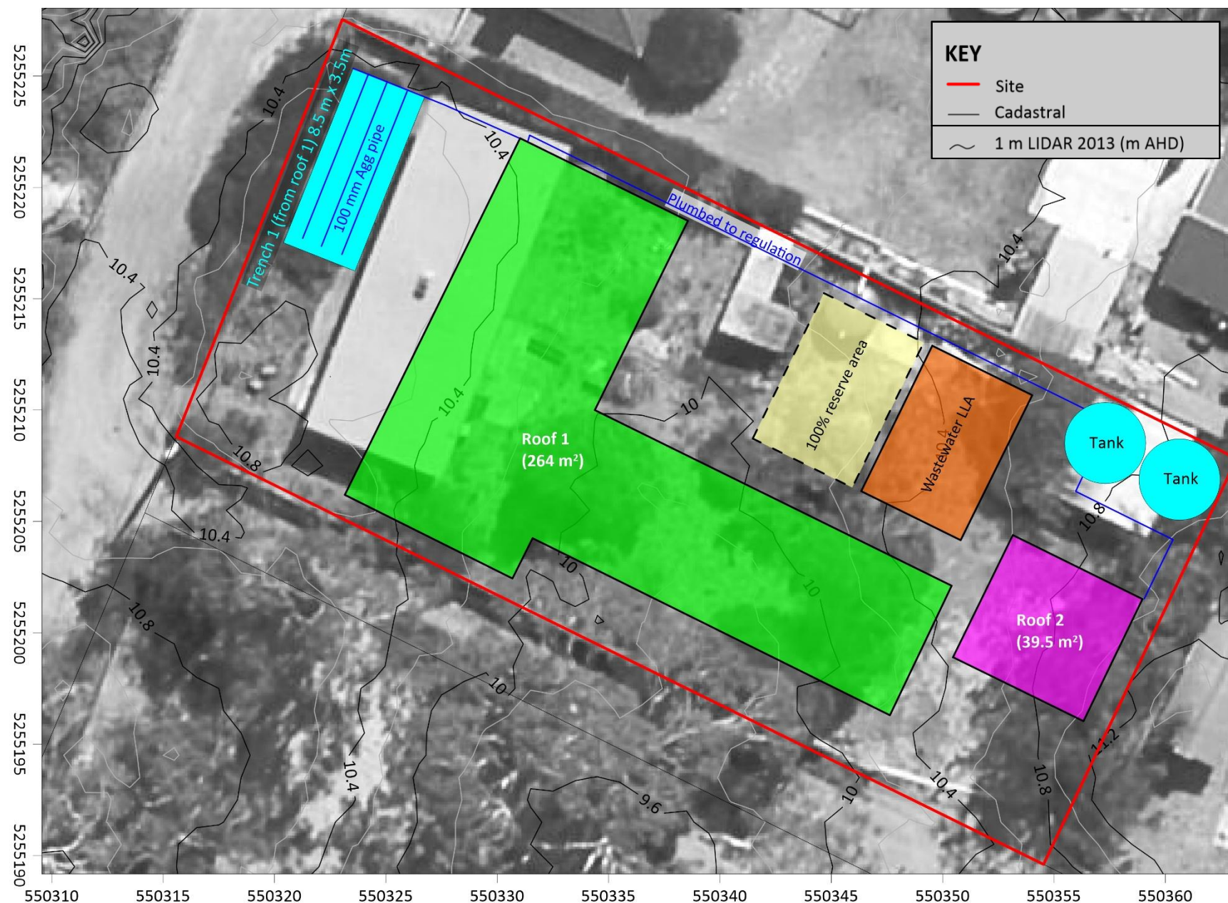
Map 2 Stormwater detention pit dimensions – refer to Attachment 2 for plumbing
