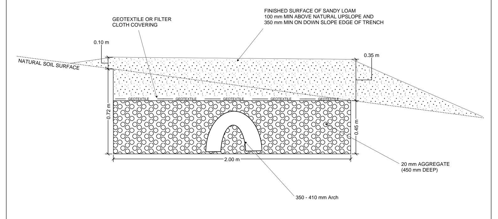
Terraced Absorption Trench Detail
