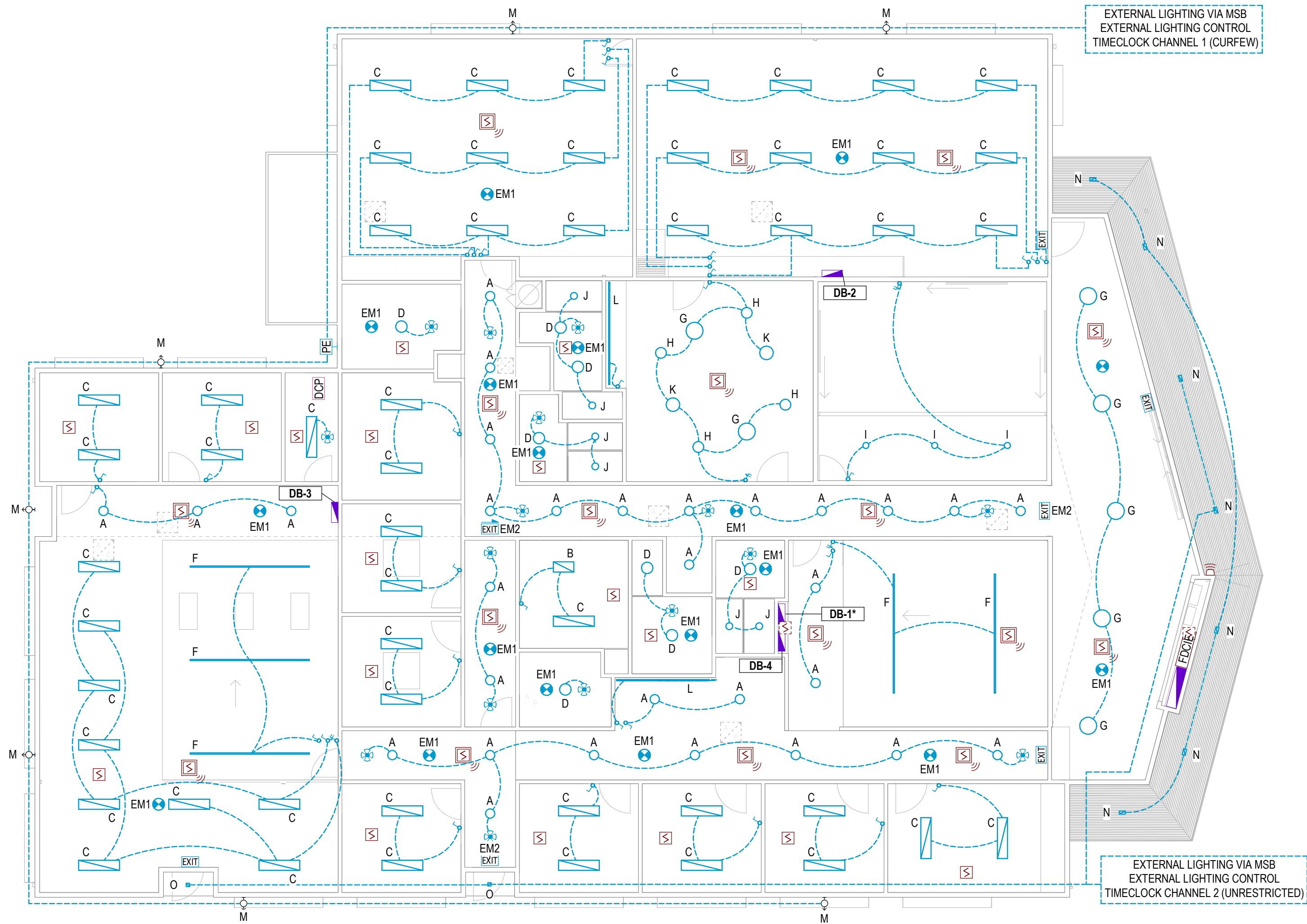
GROUND FLOOR - LIGHTING & FIRE DETECTION LAYOUT 1 : 100
