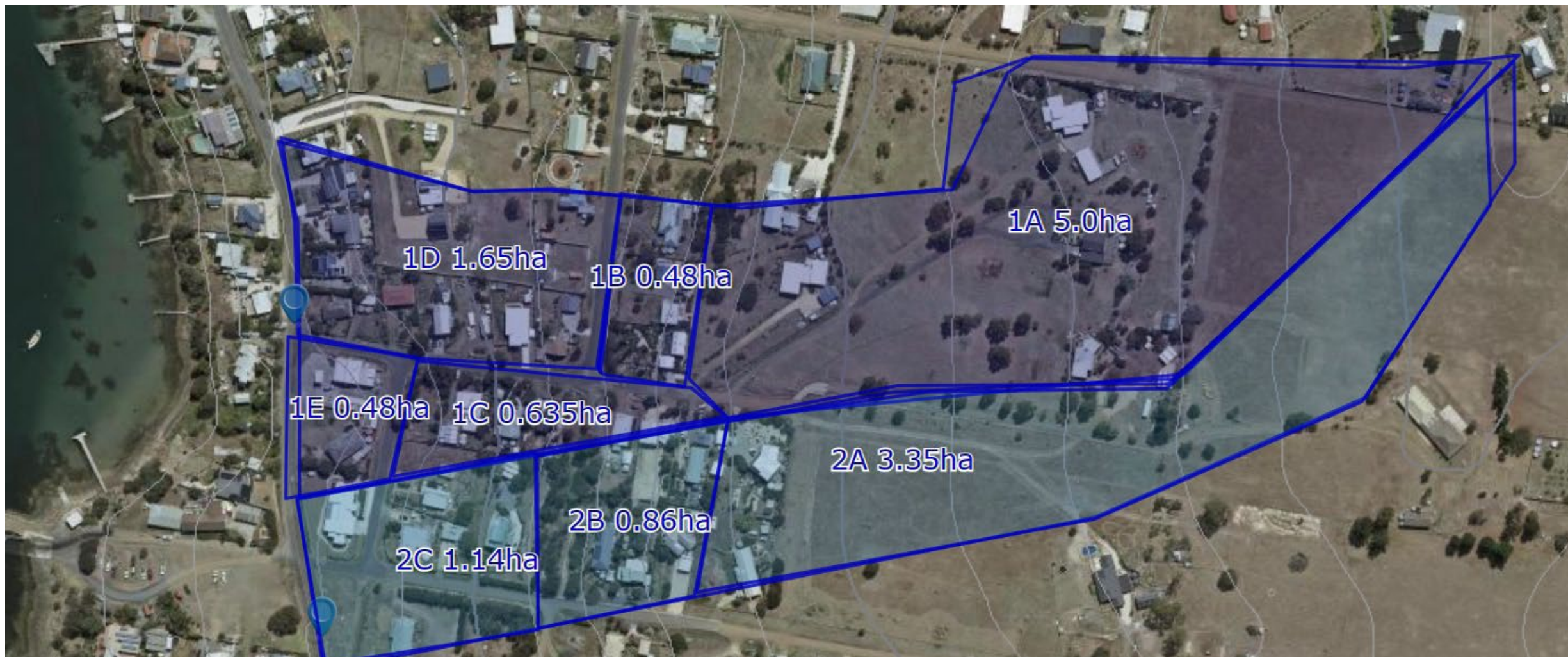
Figure 7 Catchments used in model. Catchment 1 - existing into outfall. Catchment 2 possible addition to outfall.
