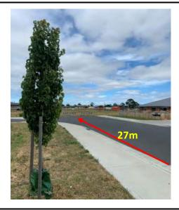
Photograph 9: Sight Distance at the basement exit was measured to be 27-metres towards the south which is not compliant.
