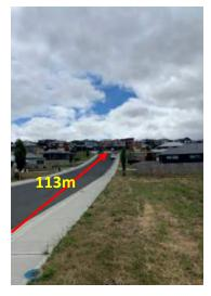
Photograph 8: Sight Distance at the basement exit was measured to be 113-metres towards the north (which is complaint with the requirements of the Sorell Interim Planning Scheme, 2015 which notably requires a sight distance of 80-metres).
