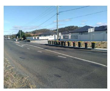
Allowance should be made for bins to be located such that there is a minimum 600mm (60cm) between each bin to aid in efficient collection by waste collection trucks. This will allow for the placement of both garbage and recycling bins, while also providing sufficient spacing for the waste collection contractor to pick up and put down bins without interfering with adjacent bins. Drivers of waste collection vehicles will not leave a vehicle to arrange or move bins.
