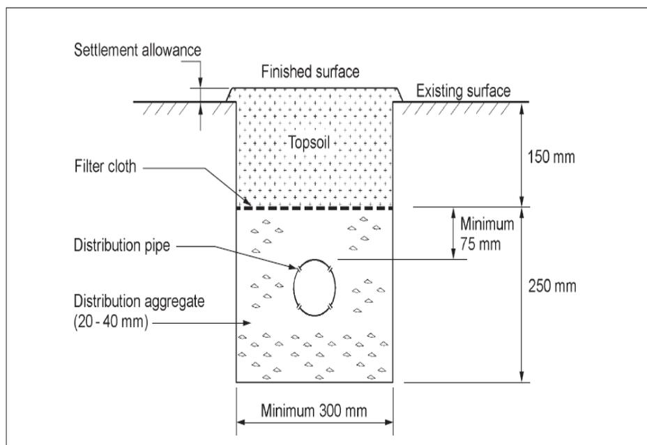
Absorption trenches will not last forever, eventually they ‘clog up’ and new absorption trenches are required. Please consult Council’s Environmental Health Officers for information on the process for installing new trenches. The length of time that absorption trenches lasts depends on:
